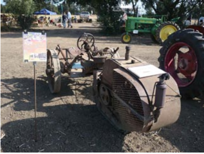
A 1937 Unitrac, Powered by a 2 cylinder Indian motorcycle Engine.
