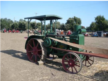
A Rumely Oil-Pull Tractor Powering one of the Threshers.
